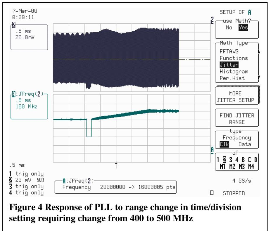
**Figure 4 Response of PLL to range change in time/division setting requiring change from 400 to 500 MHz**
