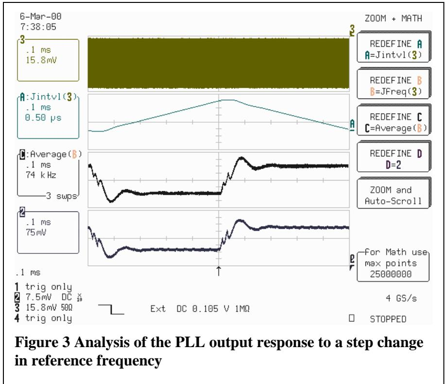
**Figure 3 Analysis of the PLL output response to a step change in reference frequency**
