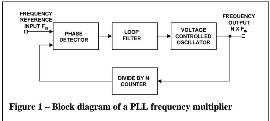
Figure 1 – Block diagram of a PLL frequency multiplier
